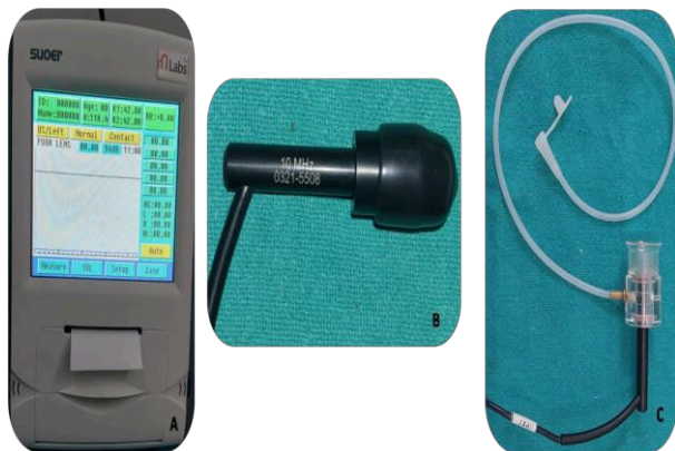
Fig. 1: (A) SuoerMlabs A-scan machine, (B) 10 MHz A Scan probe, and (C) Immersion (Scleral) shell with probe
