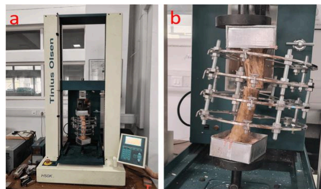
Fig. 4: 50 kN closed-loop compression testing machine showing (a) the CEF construct, and (b) the MCEF construct mounted for axial compression testing
