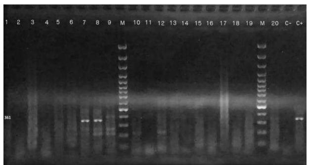
**Fig. 5:** *Mycoplasma ovipneumoniae* PCR electrophoresis analysis in 1.5% gel agarose. M: Marker (100 bp DNA ladder), Lane C+: Positive control (361 bp band), Lane C-: Negative control, and Lanes 7 and 8: positive samples of *M. ovipneumoniae*
