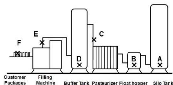
**Fig. 1: Sampling sites along the production line for pasteurized milk**
