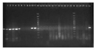
**Fig. 6:** *Mycoplasma arginini* PCR electrophoresis analysis in 1.5% gel agarose. M: Marker (100 bp DNA ladder), Lane C+: Positive control (545 bp band), Lane C-: Negative control, and Lanes 1 to 5 and 10 to 11 positive samples of *M. arginini*
