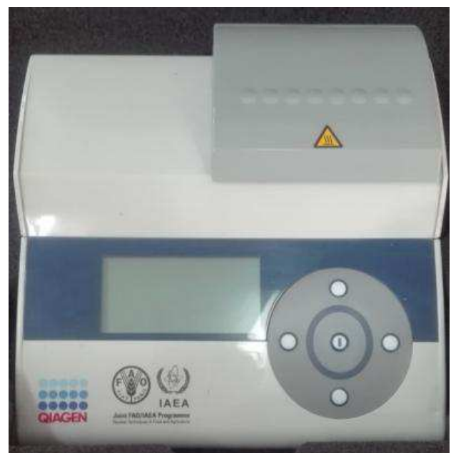
Fig. 1: ESE Quant Tube scanner. Instrument used for amplification of field samples in RT-LAMP
