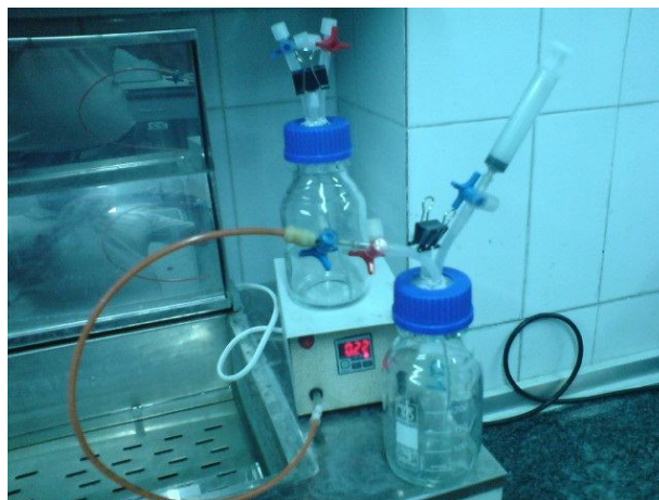
Fig. 1: A fermentation unit equipped with silicon junctions and three-way stopcock to facilitate sampling of liquid phase and measuring the amount of gas production at different times post-incubation
